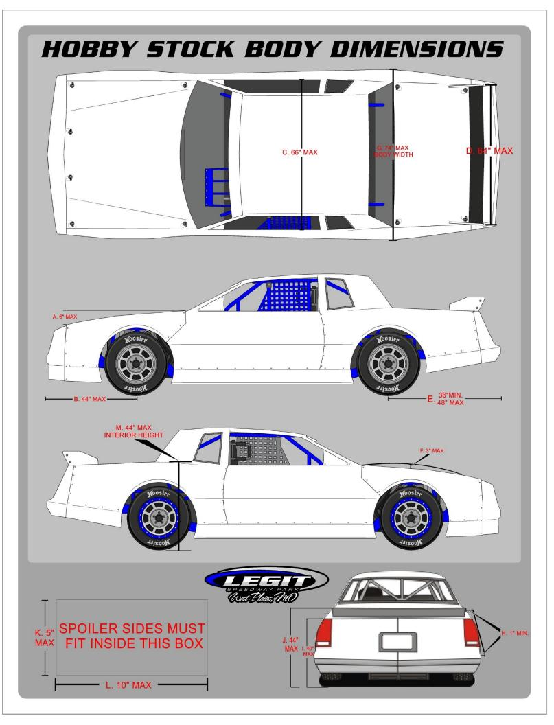
Interior deck max 40". B-post side panels must be open and resemble OEM windows stock dimension & appearance. Roof must stop 6" short of rear deck. 108" wheel base minimum. No dishing or ramping of interior deck. All other Hobby Stock Rules apply.
